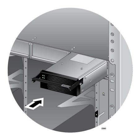
Figure 53. Inserting the AT-SBxPWRSYS1 AC Power Supply
